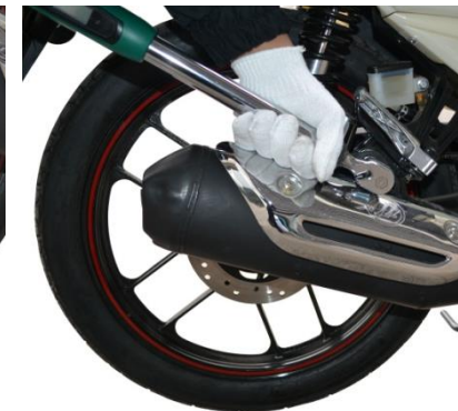
MUFFLER TIGHTENING TORQUE: 24~30N.m
