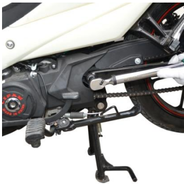
REAR FORK SHAFT TIGHTENING TORQUE: 45~65N.m
