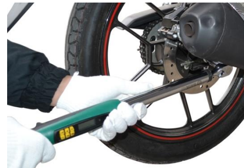
REAR WHEEL TIGHTENING TORQUE: 60~80N.m
