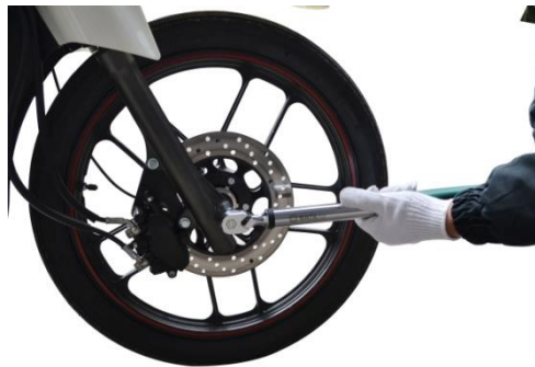
FRONT WHEEL TIGHTENING TORQUE: 60~80N.m
